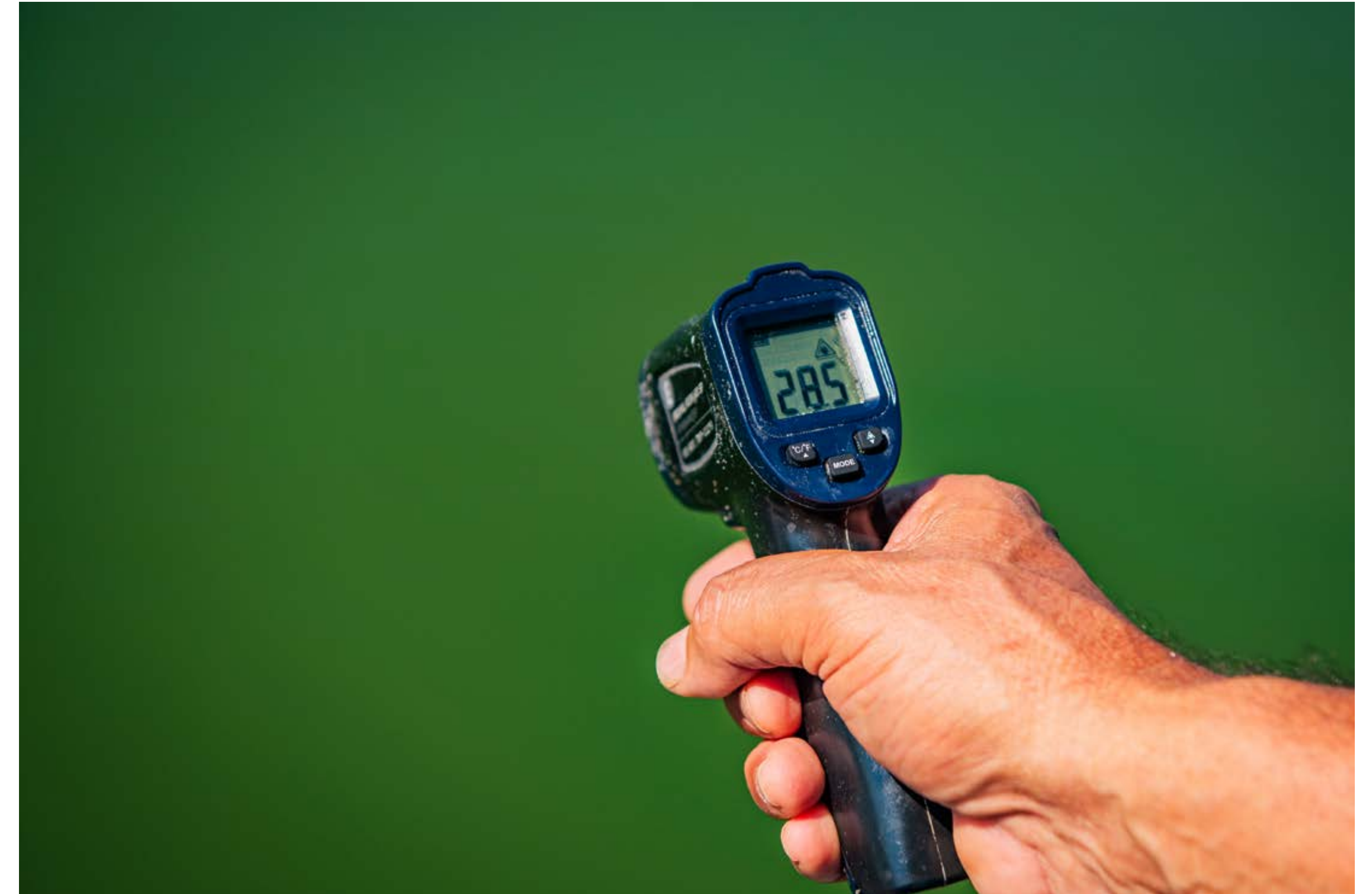
(Sacca degli Scardovari, Italy) Stefano, a mussel farmer with the Consorzio Cooperative Pescatori del Polesine, reads 28.5 degrees off the surface of his beds with an infrared thermometer, on 29 July 2026. In laboratory conditions almost no Mediterranean mussels die below 26 degrees; at 28 a fifth are dead within five days, at 30 four out of five within a fortnight, and what kills is duration as much as peak. July 2026 was the hottest month ever recorded in the Mediterranean, with a basin average of 27.07 degrees and 79 per cent of its surface under an intense marine heatwave at some point, the highest share ever measured in July. The northern Adriatic, shallow and half-enclosed, has gone from a historical summer average of 24 to 25 degrees to peaks near 30; the Mediterranean as a whole is warming at roughly twice the rate of the global ocean. In the days around this reading, the lagoon reached 32.
