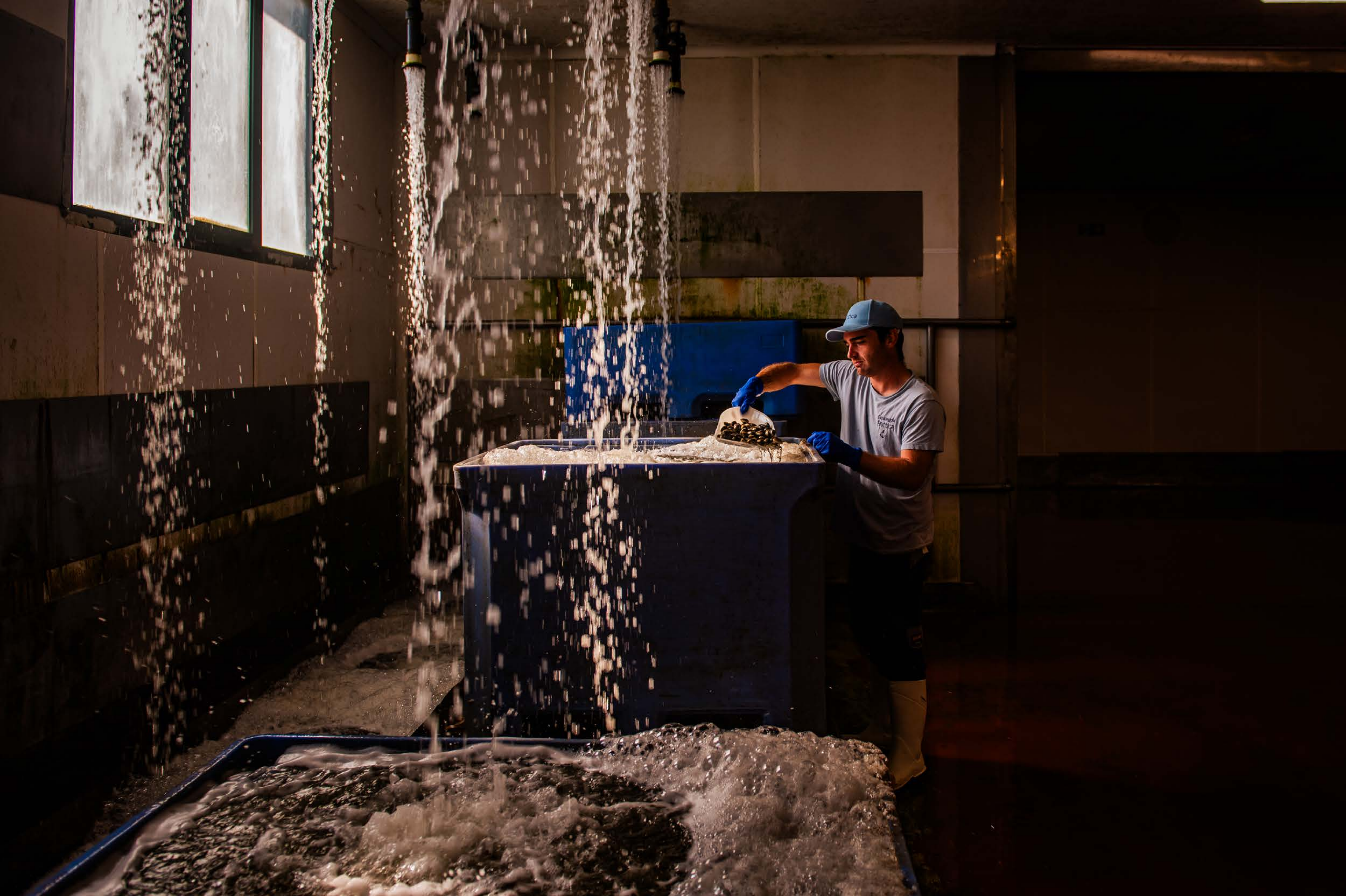
(Finittica, Goro, Italy) Clams go into the purification tanks at Finittica on 3 August 2026. Shellfish beds are graded A, B or C by the level of E. coli in the flesh: what comes off a class B bed cannot be sold until it has been through a plant like this one, where the animals sit in clean seawater and filter themselves clean, for anything from hours to days. Finittica's circuit is closed and handles more than 20 tonnes per cycle, in a plant of about a thousand square metres a few kilometres from the beds. The company was founded in 2018 by people already working in the lagoon, and follows the animals from fertilisation to packing. This summer the water outside reached around 32 degrees, growers reported losing up to 90 per cent of the clams on the beds, and what arrives at these tanks is what survived.
